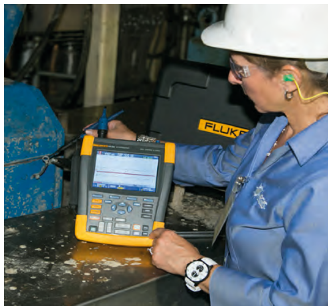
Once the AEGIS® PRO Series Bearing Protection Ring had been installed and the motor restarted, an AEGIS® technician confirmed that motor shaft voltages were minimal using an oscilloscope. A special “pigtail” lead allows maintenance personnel to periodically check the voltages (and therefore the likely condition of the bearings) safely and easily, without exposing the shaft. The ring has been diverting potentially damaging voltages to ground since it was installed.
